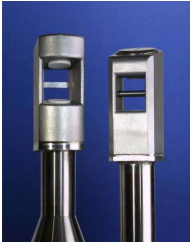
Figure 13 Vortex flow meter (picture by Höntzsch)
