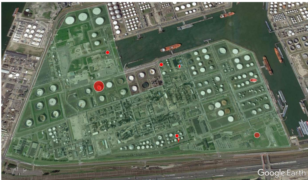
Figure 6. Local hotspots found during real-time concentration measurements using the mobile extractive FTIR, based on data in Figure 5.
