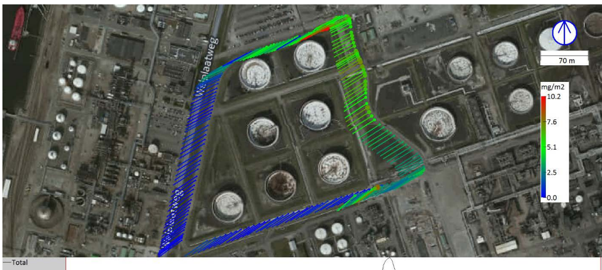
Figure 16 Example of SOF alkane transect from the West Tank Park, 2017-06-15 at 13:10. The dots show the trace of the vehicle and the color indicate the local alkane column ( \text{mg}/\text{m}^2 ) according to the color bar scale. The lines connected to the dots point in the direction of the wind.
