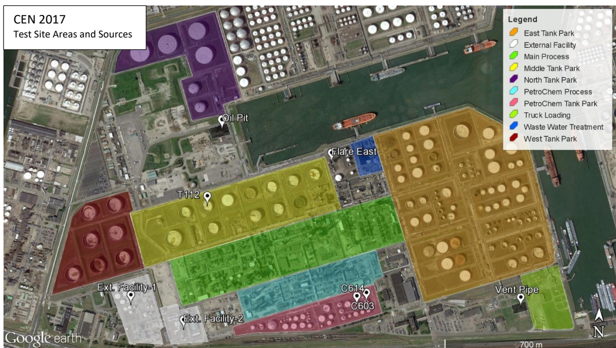
Figure 4. Map showing the measured sources of the Test Site during the CEN THE NETHERLANDS 2017 survey. Local sources are denoted as white pins and area sources as shaded regions. Map from Google Earth © 2017.
