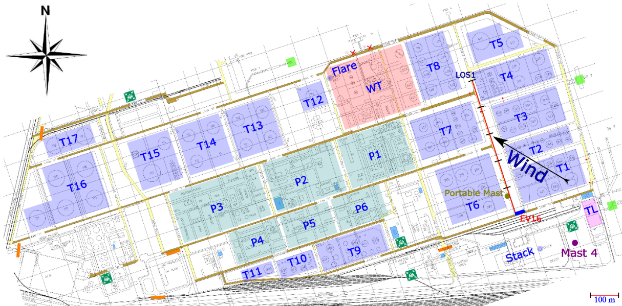
Figure 5.14 Measurement configuration for location EV16 on 14 th June.
