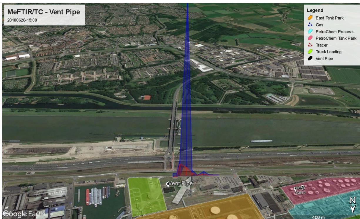
Figure 9 Alternative visualization of MeFTIR/TC measurements of the Vent Pipe, 2017-06-20 at 15:00. The height of the blue line is proportional to the ground level concentration of Butane equivalents (1 m is equivalent to 1 ppb; max measured value was 906 mg/m 2 ) and the red line is proportional to the ground level trace gas concentration (1 m is equivalent to 1 ppb; max measured value was 81 mg/m 2 ). Different areas of the test site are shown as colored fields. The wind direction is indicated by the white arrow. Map from Google Earth™ 2018.
