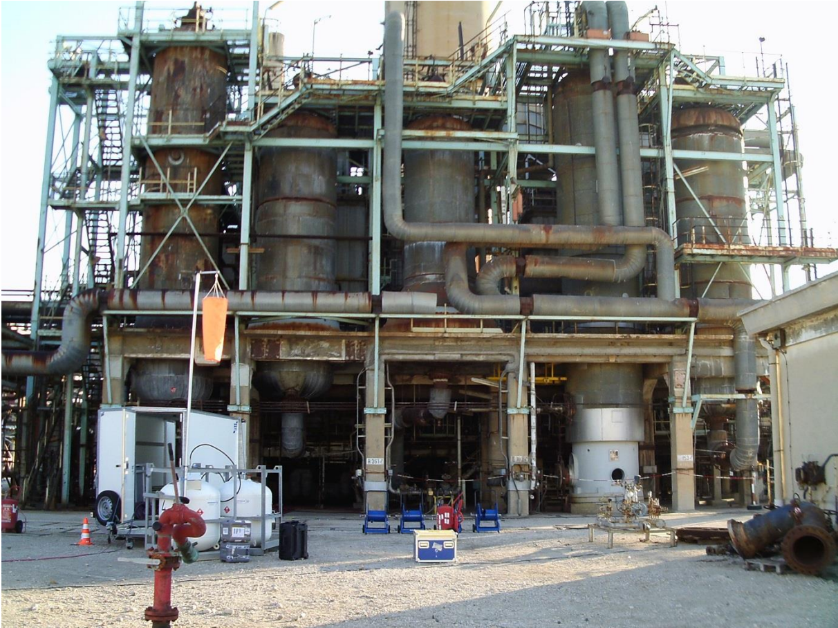
Figure 5.3. Photograph of controlled release arrangement with propane tanks and CRF trailer in foreground and unit where release nodes were positioned in background.
