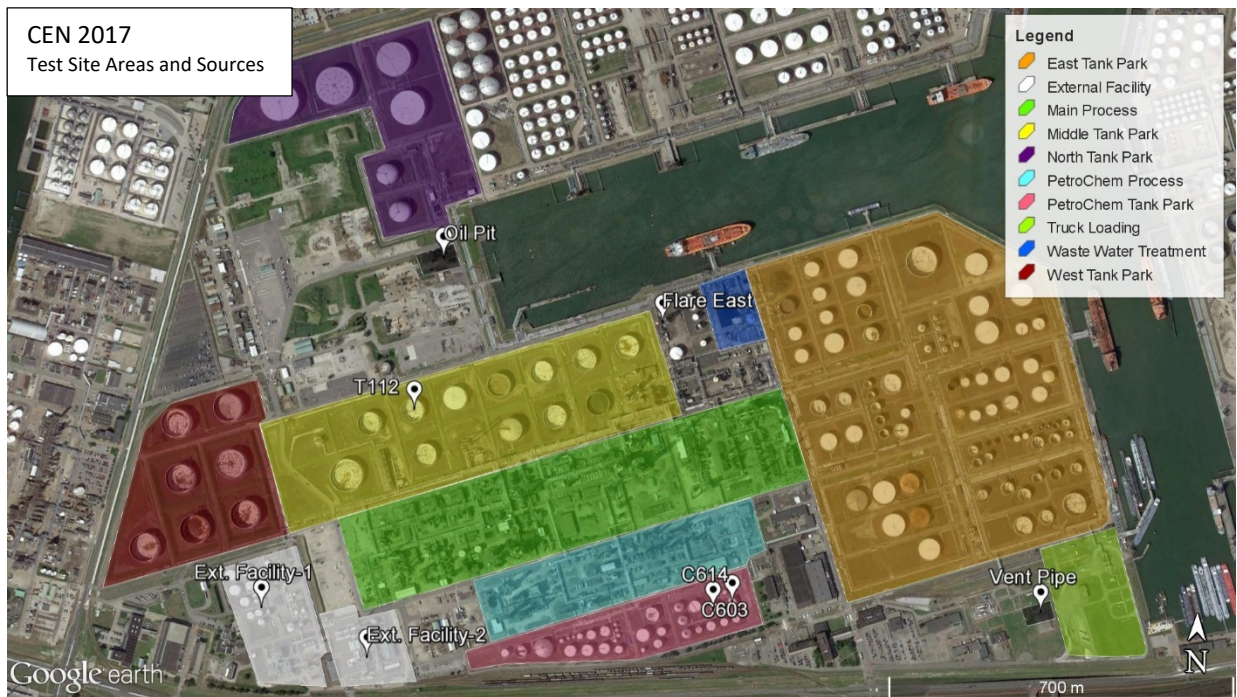
Figure 3. Map showing the measured sources of the Test Site areas during the CEN THE NETHERLANDS 2017 survey. Local sources are denoted as white pins and area sources as shaded regions. Map from Google Earth © 2017.
